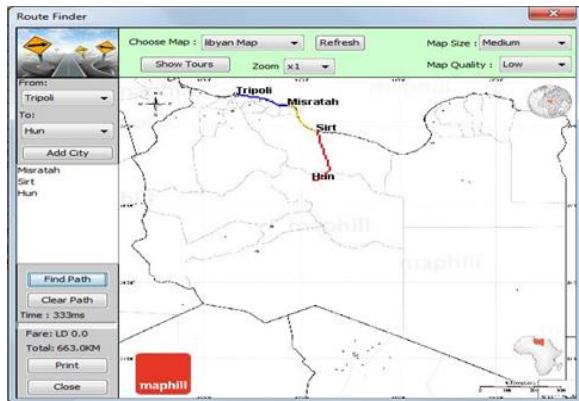
Figure (7) The output of calculating the time and path using the algorithm (A*)
